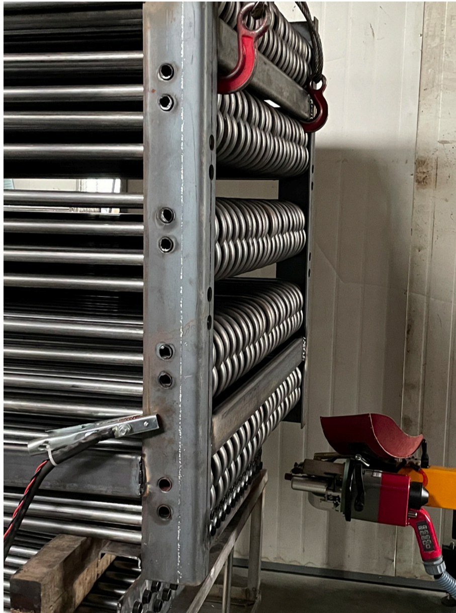
STAINLESS STEEL 304 COIL Laser Welding
