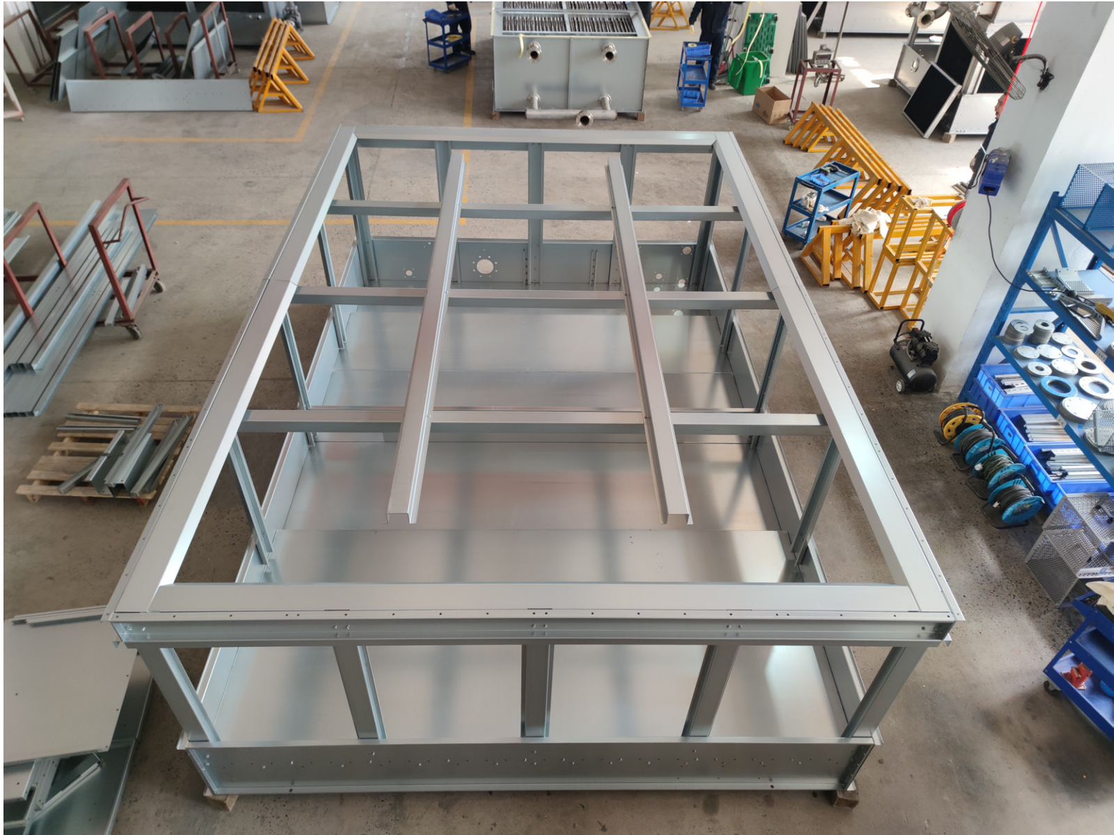
Galvanized Steel Casing Zinc Coated 700 gr/m 2
