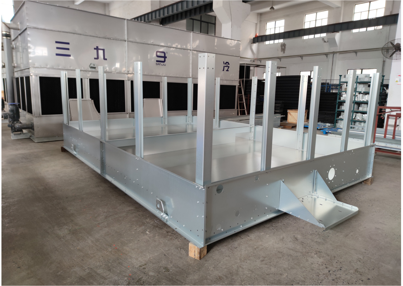
Galvanized Steel Casing Zinc Coated 700 gr/m 2
