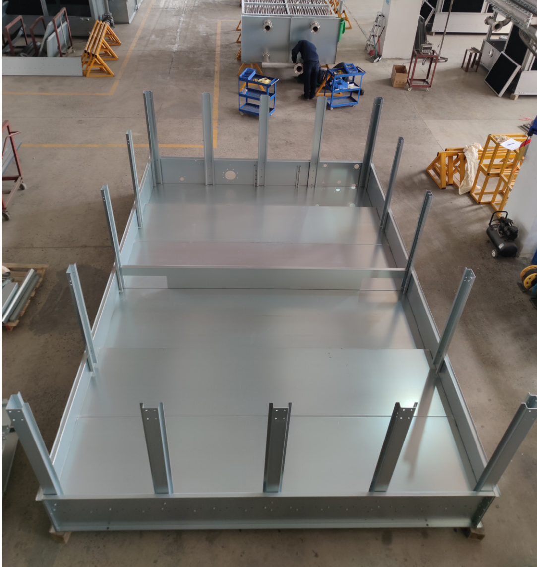
Galvanized Steel Casing Zinc Coated 700 gr/m 2
