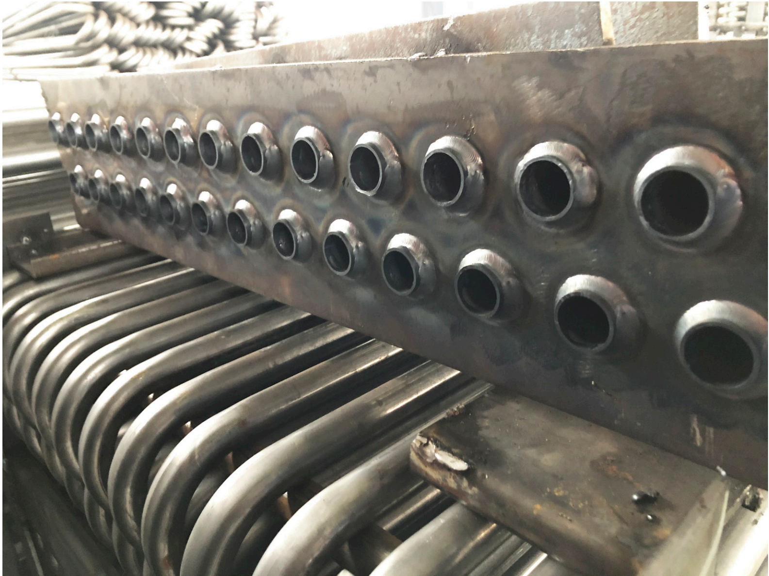
STAINLESS STEEL 304 COIL Laser Welding
